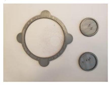
In Figure 7, two copies of the fully printed shape from Figure 5 and 6 are displayed along with their 3D printed counterpart. These objects were printed with Poly-Lactic Acid (PLA) plastic, a durable, non-toxic, and beginner-friendly material. Looking closely, one can see striations on the objects, a result of the of how the strands of plastic are thinly layered and deposited by the printer nozzle.
